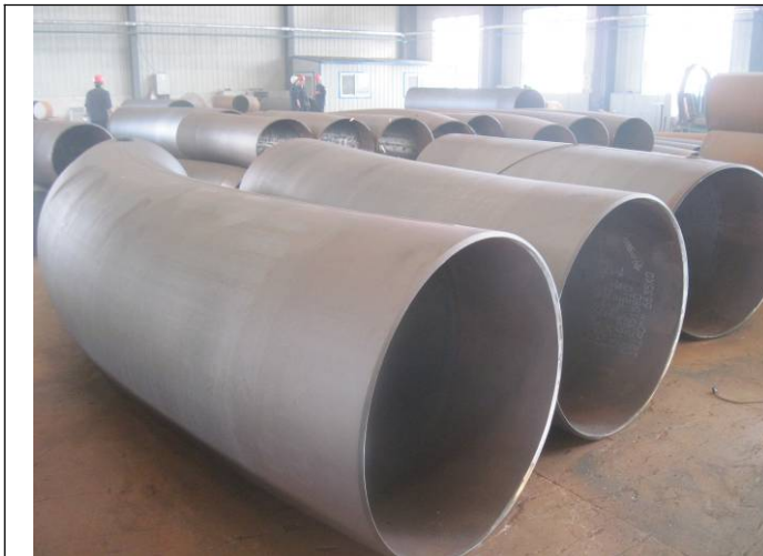
Bends after being abrasive blast cleaned
