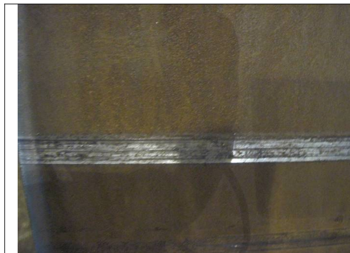
Severe machining mark
