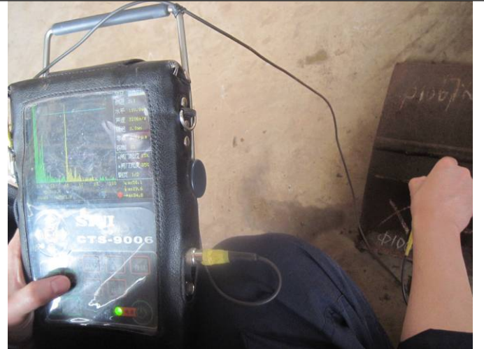
UT equipment 3 calibration
