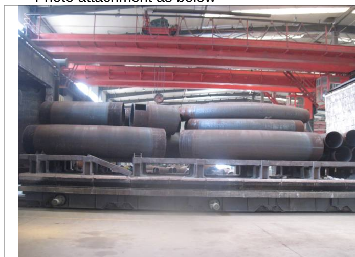
Bends in the furnace
