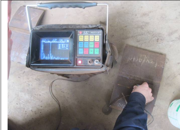
UT equipment 2 calibration
