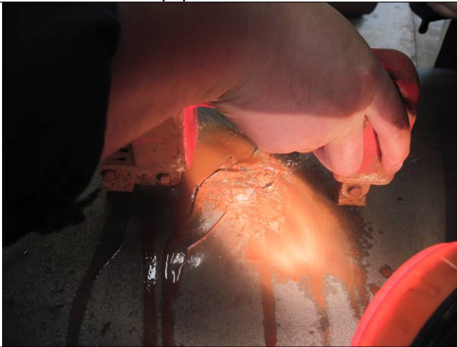
MPT equipment calibration
