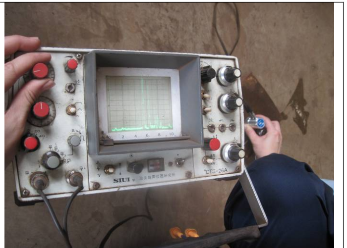
UT equipment 1 calibration
